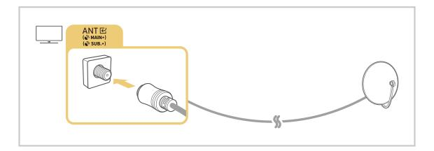
It is best to connect the both connectors using a Multi-Switch or DiSEqC Switch, etc and to set Aerial Connection Type to Dual.
