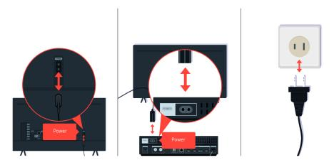
First disconnect and reconnect the power cables and HDMI cables on the back of your TV or the One Connect Box, then unplug the power cable and plug it back into the wall outlet.
