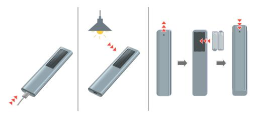
If you cannot see infrared signals, charge the remote control by using the USB port (C-type) on the bottom, or turn over the remote to expose the solar cell.
